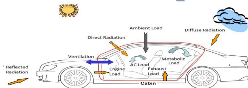
Figure 1: Various thermal load
